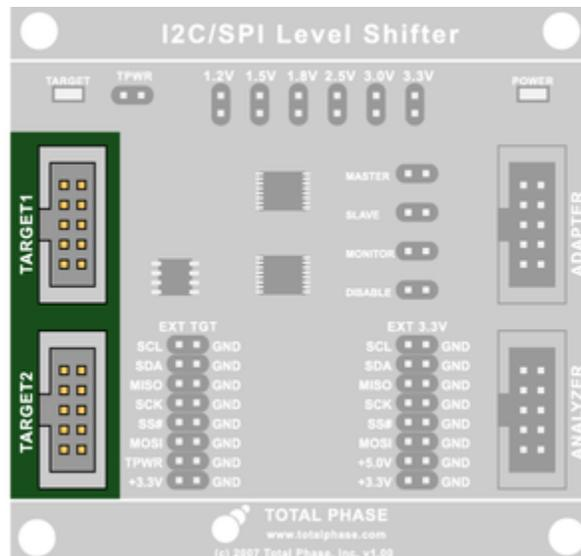
**Figure 5 :** Two boxed connectors for connecting the Level Shifter Board to one or more target buses.
