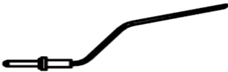
**Z-Ground:** The Z-Ground is designed to be attached to either socket of the probe head. The Z-Ground is the highest quality grounding solution and is recommended in high frequency applications.
