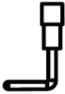
**L-adapter:** This adapter has a socket on one end and a square pin with a right angle on the other to connect to the input or ground socket of the probe body, and may be used for high frequency applications.
