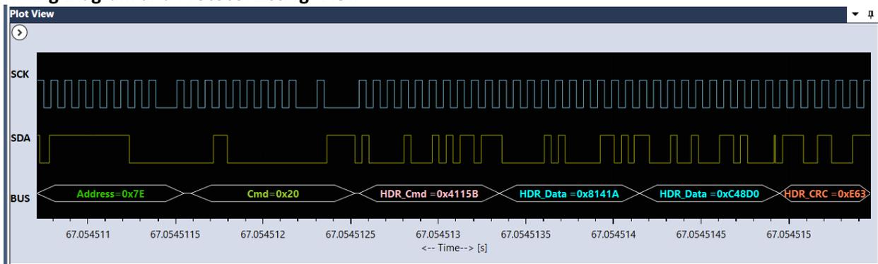
Timing view provides the plot of SCL and SDA signals with bus diagram. Overlaying of Protocol bits on the digital timing waveform will help easy debugging of Protocol decoded data. Cursor and Zoom features will make it convenient to analyze Protocol in timing diagram for any timing errors.
