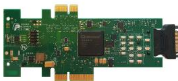
PCIe Test Card with Molex to SATA Adapter Attached
