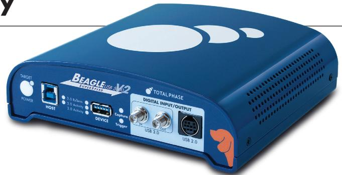
tedious and time-consuming. However, if there is an error in either the enumeration or the transmission of data, the Beagle USB 5000 v2 analyzer and its real-time analysis feature is uniquely suited to provide the visibility and immediate feedback to the user.
