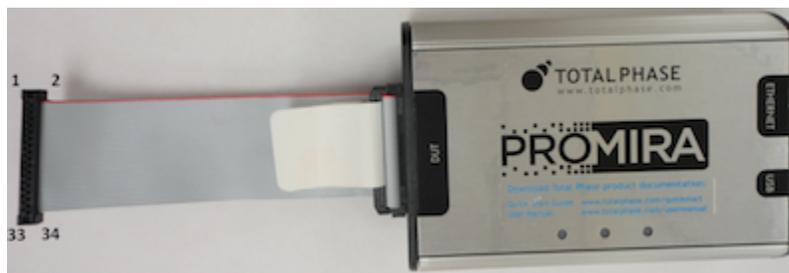
**Figure 11** : Promira platform front position with 34-34 cable
