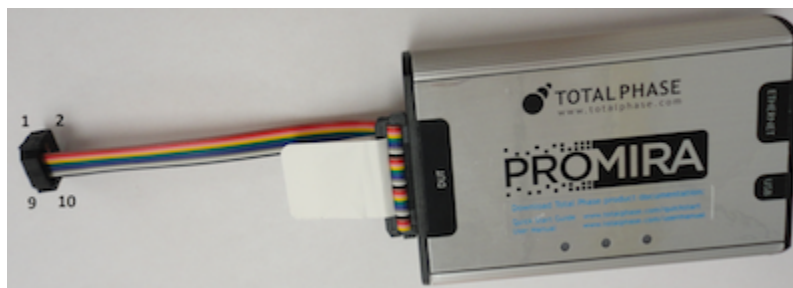
Figure 5 : The Promira platform front position with 34-10 cable.
