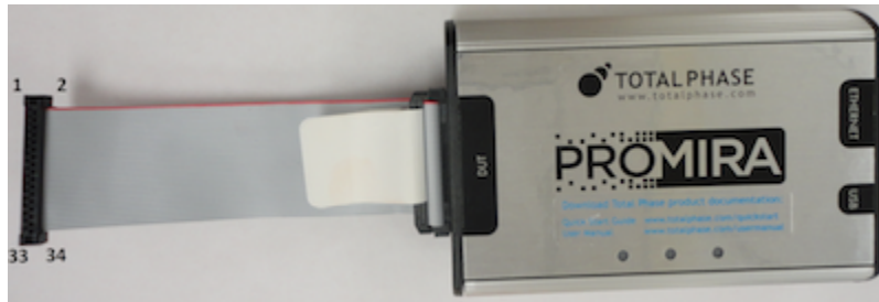
Figure 6 : Promira platform front position with 34-34 cable
