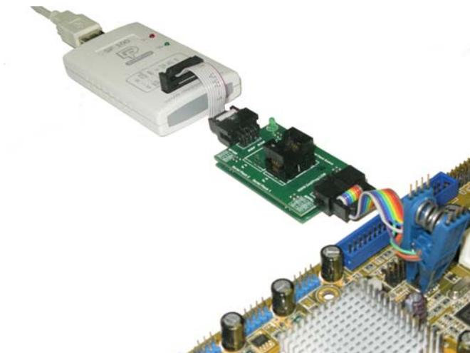
**Useful for the Bios repairing if ISP method is not supported:**
