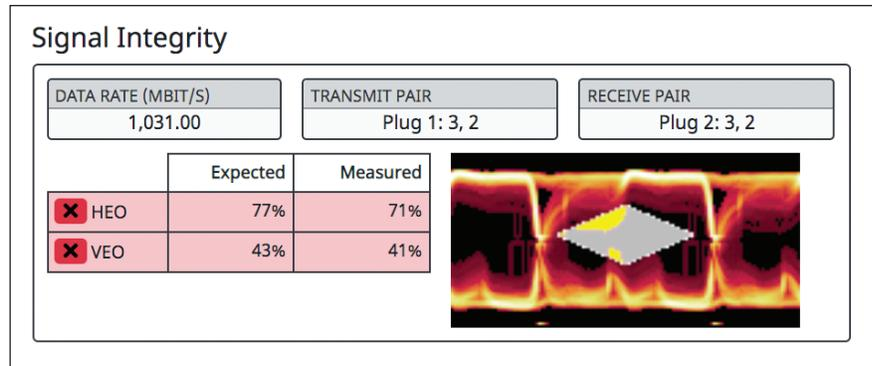
Figure 3. Test results extract of Signal Integrity for a USB Standard-A to USB Standard-B Cable.
