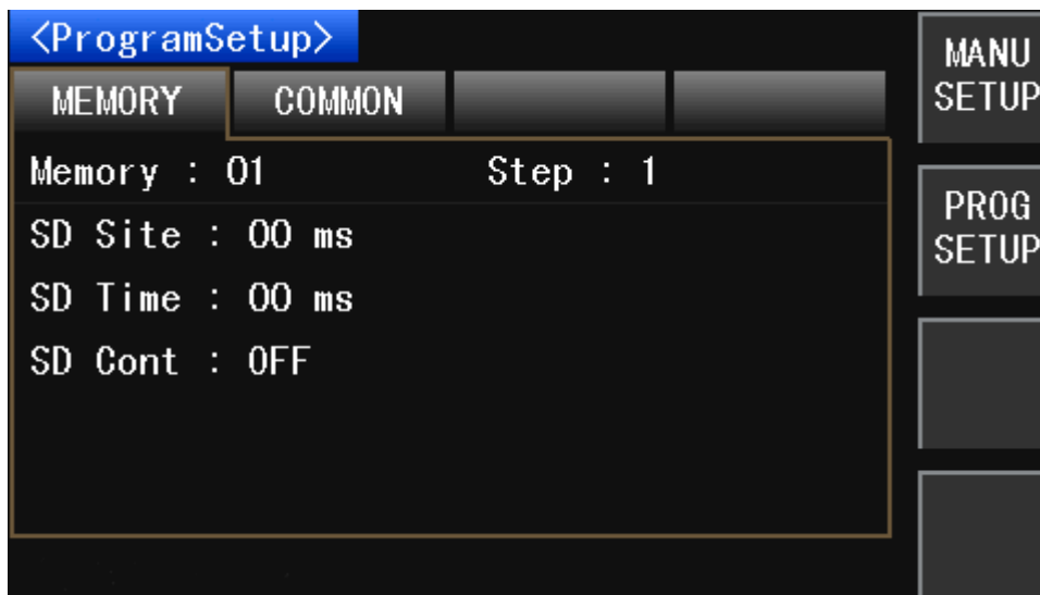
Figure 3-12 Sequence setting page 3 in <programmable mode>
