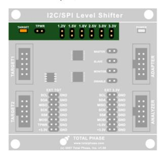
**Figure 10**: A jumper must be placed on the appropriately labeled header for the desired voltage level. If supplying power from the Level Shifter Board to the target, a jumper needs to be place on TPWR as well.
