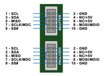
**Figure 4**: The pinout for the two boxed connectors on the Adapter/Analyzer side of the Level Shifter Board.
