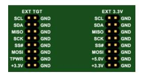
**Figure 7**: The External Connectors provide the developer with a quick and easy way to interface or monitor any or all of the Level Shifter Board signals on either the Adapter/ Analyzer side or the target side.
