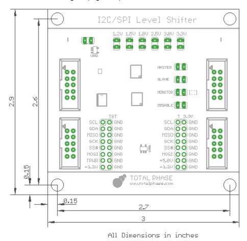
Figure 2: Dimensioned Level Shifter Drawing
