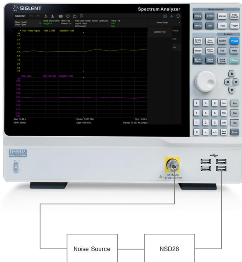
Figure 1-2 Connection setting of noise figure measurement calibration
