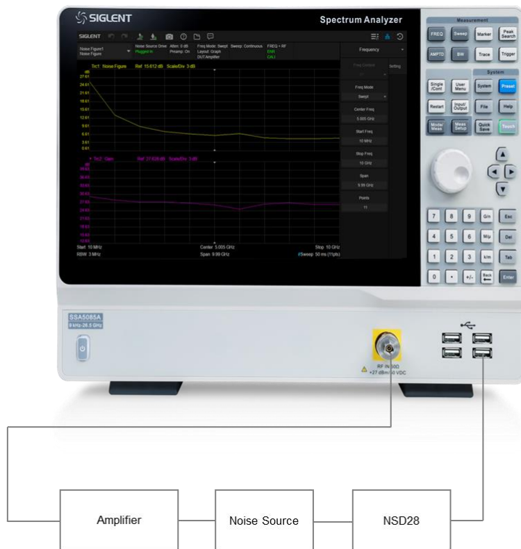
Figure 1-6 Connection settings for noise figure measurement
