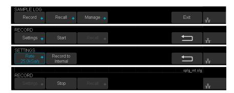
In order to reduce the amount of data logged and speed up the logging, the log file is recorded as binary, and the file name is \*.slg.
