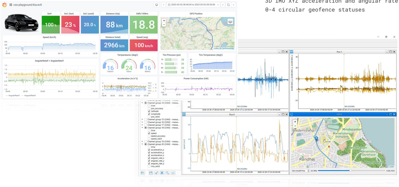
The CANedge units with GNSS/IMU are ideal for vehicle telematics, diagnostics and analysis - with easy visualization in e.g. Grafana or asammdf
