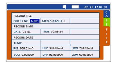
2. Use the key ( ) to select the memory number to be read out. Use the key ( ) to locate the memory number The measurement values for the selected memory number are displayed.
