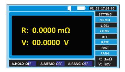
Manual range switching is effective even when the automatic range function is turned on (the automatic range function is automatically turned off when the automatic range function is turned on and the manual range function is turned off when the automatic range function is turned on) At the measuring interface, press the [AUTO] key to switch the automatic range.
