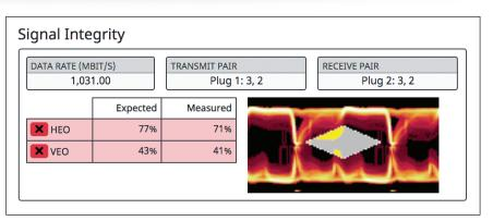
Figure 3. Test results extract of Signal Integrity for a USB Standard-A to USB Standard-B Cable.
