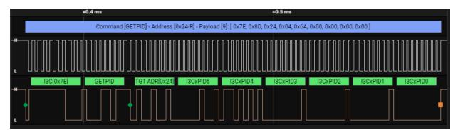
I3C Basic<sup>SM</sup> Protocol Analyzer Plugin for Saleae Logic
