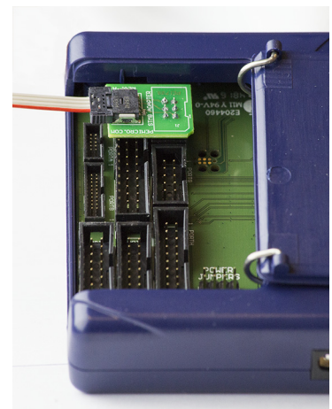
Figure 3-27: STM8 Adapter: 1) Bottom, 2) Top, 3) Connected To 6-Pin Header of Cyclone_Universal (Adapter Sold Separately)
