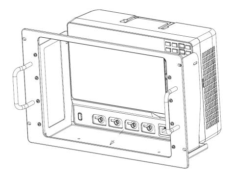
5. Use the T10 Torx driver to remove the outside top two screws from the back of the oscilloscope body.
