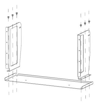
3. Attach the handles to the front plate using four M5x10 Phillips screws, then attach the front plate to the side plates using eight M4x10 Philips screws.
