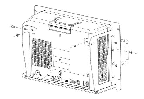
7. Post-installation notice: the rack mount occupies a height of 7U, The holes pointed out by the arrows are installation holes. They should be aligned during installation.
