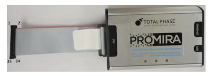
Figure 11 : Promira platform front position with 34-34 cable
