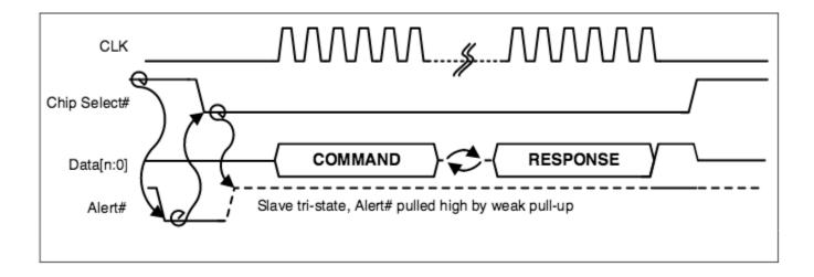
Figure 7 : Slave Triggered Transaction (Multiple Slaves)
