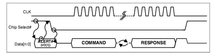
Figure 6 : Slave Triggered Transaction (Single Slave)
