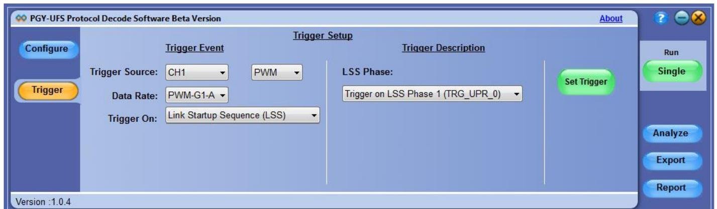
PGY-UPRO/LLI/UFS software provides protocol aware trigger conditions such as link start-up sequence, PHY adapter layer content and data link layer content. The unique capabilities in this software allow trigger data type such as PWM, NRZ or 8B/10B serial data of the protocol. PGY-UPRO supports following Protocol Aware Trigger capabilities.
