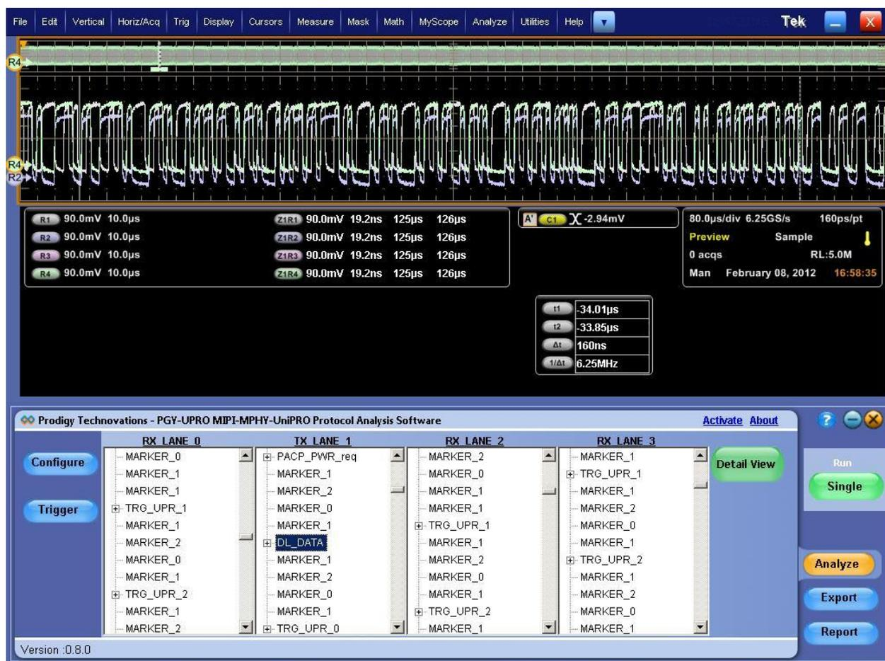
PGY-UPRO/LLI/UFS runs inside the Tektronix oscilloscopes and decodes protocols and displays the decoded data of multiple lanes. This software links the decoded data to the electrical signal in the oscilloscope display. UniPRO/LLI Protocol-based trigger can be set up using the built-in high speed serial trigger capabilities in Tektronix oscilloscopes.
