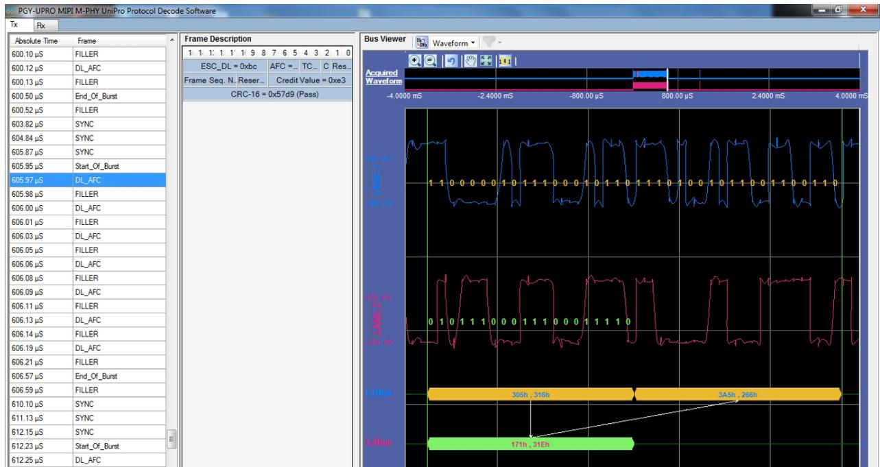
In an emerging technology, engineers test and debug UniPRO/LLI/UFS designs with easy-to-use instruments such as oscilloscopes. But oscilloscopes normally provide extensive details about electrical characteristics of the signal. But engineers need more information such as protocol content at different protocol layer. Manually interpreting the protocol layer information using oscilloscope data is time consuming and prone to human error.
