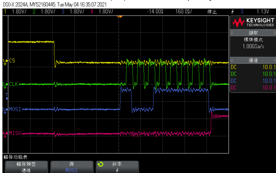
Figure: The Read ID Command of MOSI output measured by the oscilloscope is 9F, and the waveform is correct.
